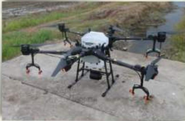
The application of a drone for foliar spraying
